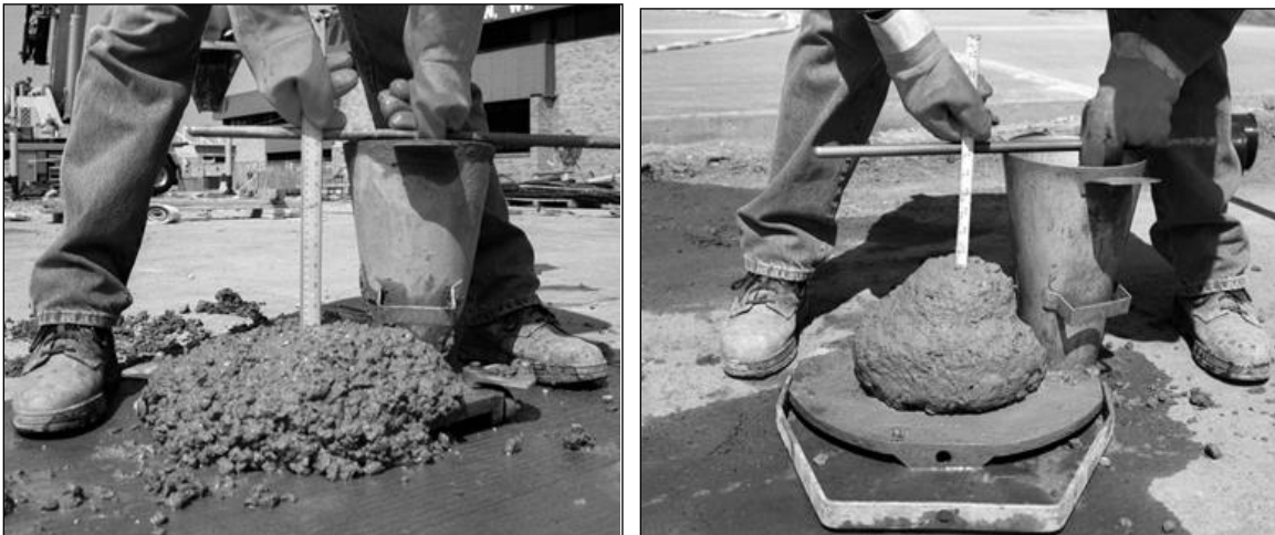
Figure 7. Slump test (left: High slump; right: Low slump)
